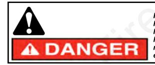
Hydraulic oil under extremely high pressure. Do not use hand or any other skin to check for or to stop hydraulic leaks. Be sure pressure is relieved before loosening hydraulic fittings. Replace worn hoses immediately. Seek medical care immediately if hydraulic oil is shot into the eye or the skin.
