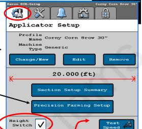
Check the **Height Switch** box if you are using a Mercury Switch or Finger Style Switch for Implement Height Indication.
