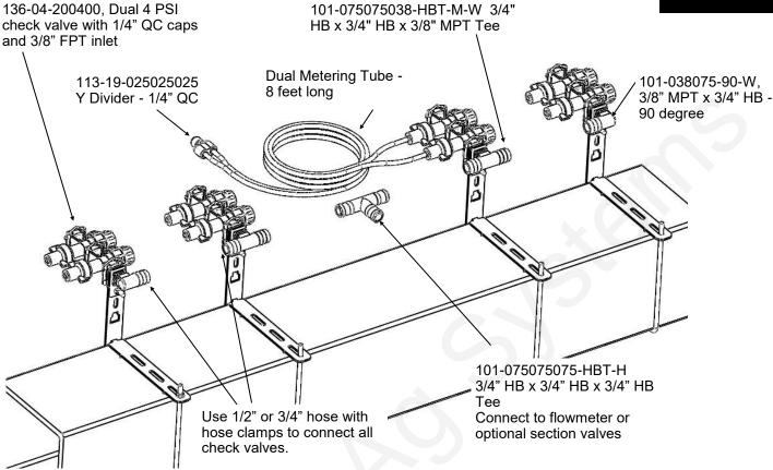
This is a general diagram showing the dual check valve assembly mounted on a planter toolbar. The check valve and bracket are very flexible in their mounting. The check valve can mount behind, directly over, or in front of the toolbar. The check valve can be put in the bracket facing up & down or sideways (shown). In addition the steel bracket could be rotated 90 degrees and clamp around the bar. The multiple slots in the bracket are used to mount to any tube 7x7 inches or smaller.
