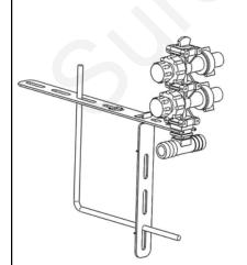
The check valve is mounted over the top of the bar. The supply line would run above and behind the bar. The short bracket is placed the notch to mount the check valve closer to the bar.
