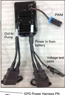
205-3118Y1 (20 feet) - connect to tractor battery.
