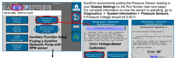
16. If using a Pump RPM sensor on a SureFire PumpRight Hydraulic Pump
