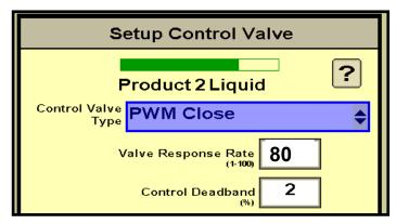
Start with the Valve Response Rate at 80. You will also make some changes in the Advanced Tuning (described later). If system is too slow to adjust to speed changes, increase Valve Response by 10 at a time.
