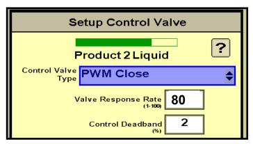
Start with the Valve Response Rate at 80. You will also make some changes in the Advanced Tuning (described later). If system is too slow to adjust to speed changes, increase Valve Response by 5 at a time.
