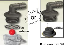
If using a metering orifice in the flow indicator, the orifice replaces the ball retainer. If not using an orifice here, the ball retainer must be in place. Remove top fitting of each column. Then push metering orifice into bottom of each outlet fitting. (This is not used very often.)
