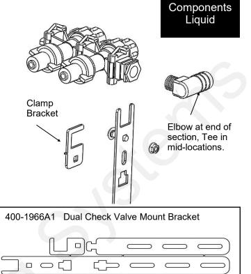
The long, short & clamp bracket come as one part connected by break-off tabs.
