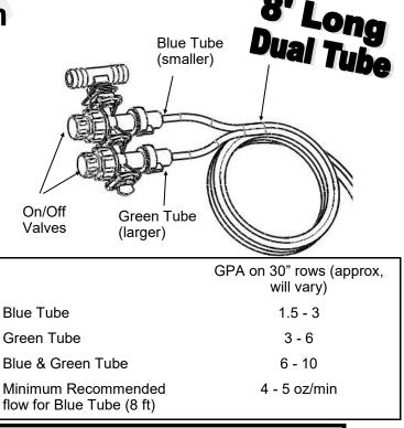
\*\* Ultra Low Rate Application –For rates from 2-5 oz/min/row use a <u>12 foot</u> length of metering tube. To calculate oz/min/row: Oz/min/row = (GPA x MPH x spacing (inches)) ÷ 46.4
