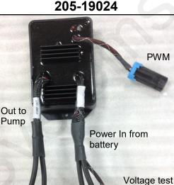
EPD Power Harness PN 205-3118Y1 (20 feet) **connect to tractor battery.** This is 6 AWG wire.
