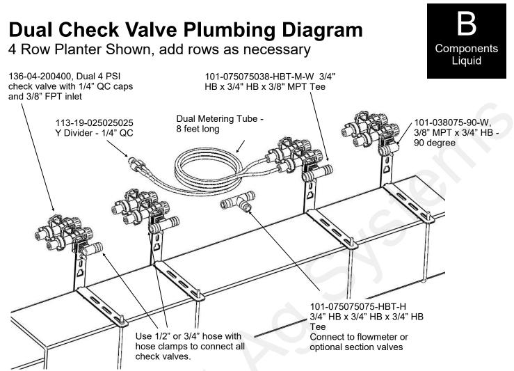
This is a general diagram showing the dual check valve assembly mounted on a planter toolbar. The check valve and bracket are very flexible in their mounting. The check valve can mount behind, directly over, or in front of the toolbar. The check valve can be put in the bracket facing up & down or sideways (shown). In addition the steel bracket could be rotated 90 degrees and clamp around the bar. The multiple slots in the bracket are used to mount to any tube 7x7 inches or smaller.
