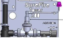
Pressure Sensor (3 wire type) with harness 521-05-050150
