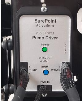
The **Green Power light** should be on when the EPD is receiving power from the battery.
