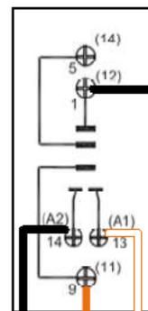
*If the Pivot Kill Output connector is unplugged from the controller or the controller power is off, the Pivot Kill signal will be in bypass.*
