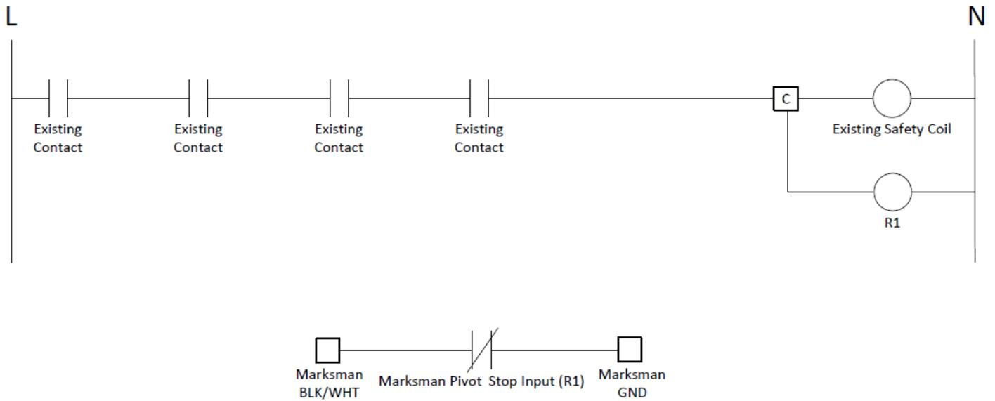
Marksman Pivot Stop Input (R1) coil connection (Connection C) can be placed anywhere where there is 110VAC when the Marksman is permitted to run. This is an example of a circuit.
