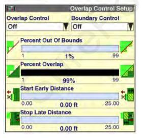
Overlap Control and Boundary Control must be ON for automatic section control on overlap and boundaries.
