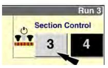
The number of sections available is determined by the planter type. Liquid application sections must match planter seed sections.
