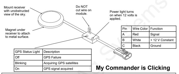
ISSUE: Controller goes back and forth quickly and repeatedly from RUN to HOLD. Controller has a fast clicking sound (1) when I start driving or (2) when I start applying.
