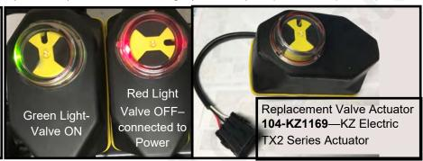
This is a 3-way valve. If product will not flow when valve is ON, either move the outlet hose to the other outlet port, or remove actuator and rotate valve ball 180°, and replace actuator. Product should flow
