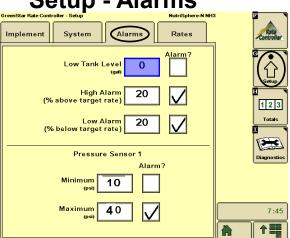
Low Tank Level can be set if desired. Tank level will be measured in ounces, not gallons.
