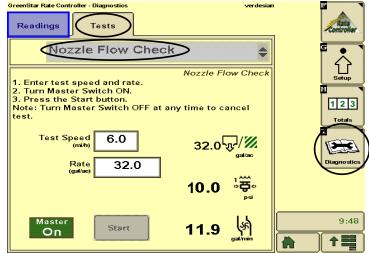
Use Nozzle Flow Check to see if system will lock on to a rate at a test speed. Pressure with water will be a lot lower than it will be with a heavier, thicker product.
