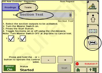
Section Test can be used for manual operation of the system. It can be used to prime the pump on startup or to rinse the system. It is good for troubleshooting.
