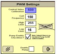
Change first digit of Control Valve Calibration to speed up or slow down control changes.
