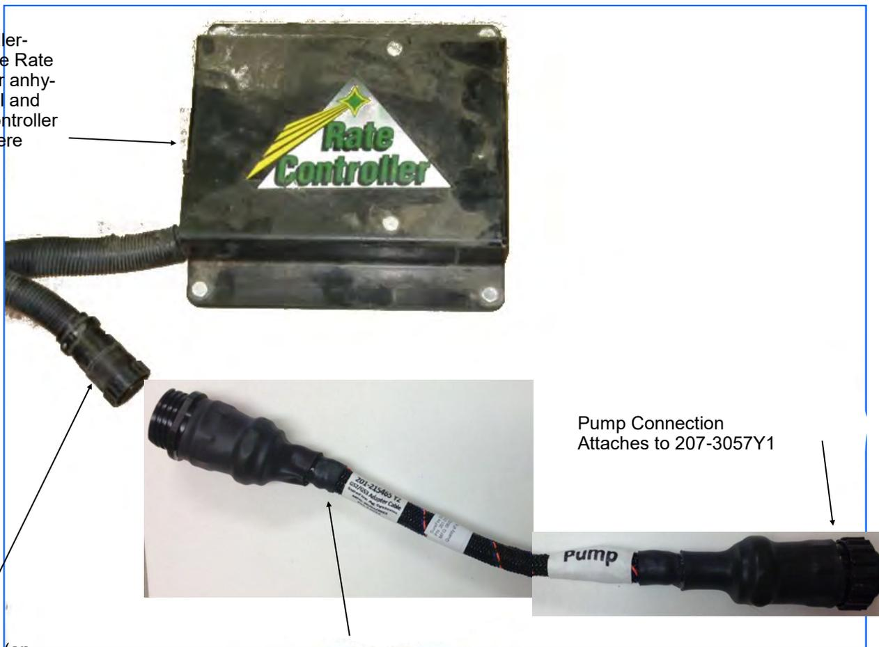
37 Pin Connector (on John Deere Harness)
