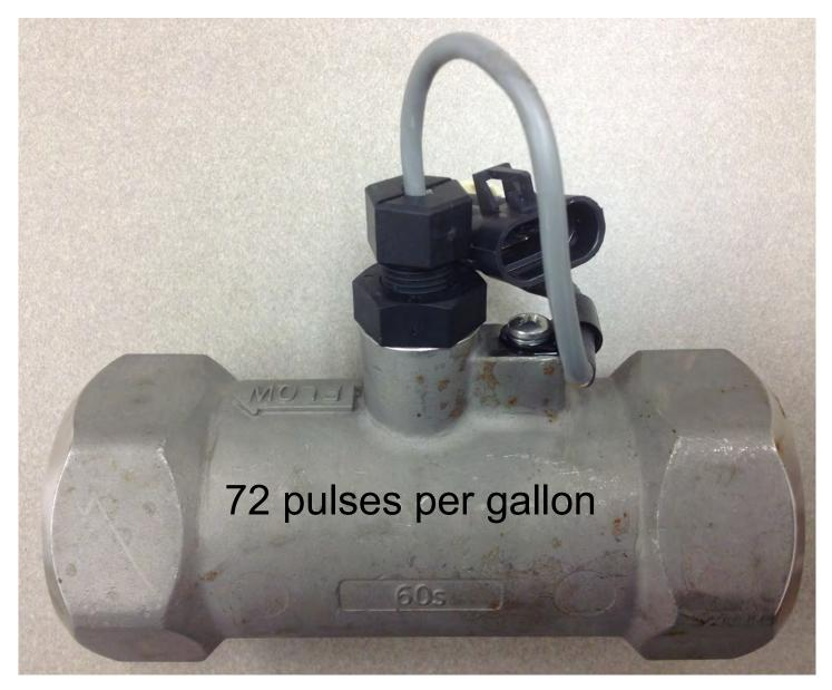
The flowmeter calibration number is **72 pulses per gallon**. Verify accuracy of flowmeter by comparing the Volume shown on the display with actual weigh tickets. If the weigh ticket amount is more than shown on the display, LOWER the flow cal number. Use the following formula to adjust the flow cal number:
