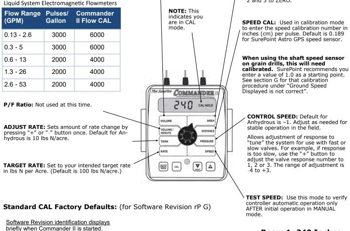
Anhydrous Flowmeter VOLUME AREA FLOW 72 pulses/gal VOLUME/ **P/F RATIO** DISTANCE Off MINUTE ADJUST TANK PRESSURE 10 lbs N/acre RATE 100 lbs N/acre RATE SPEED TARGET
