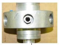
Threaded orifice installed
