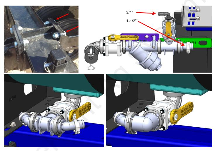
3. Plumbing for under the tanks is assembled as shown above. The front tank is shown on left, rear tank is on right. Reference Bill of Materials on page 3 as necessary. Begin by threading plug into bung that will not be used. Thread Manifold x MPT fitting into other tank bung individually. Assemble tank outlet manifold fittings as shown. Route 1-1/2" hose through slots in tank saddles for support.
