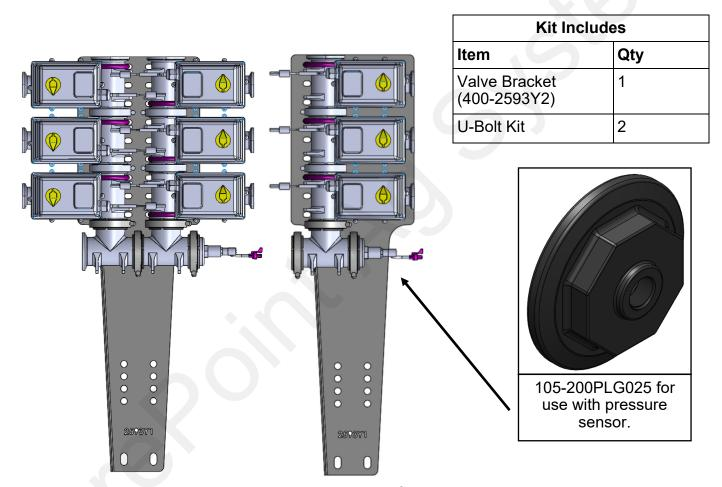
Recommended double- and single-stack orientations for Banjo Section Valves.
