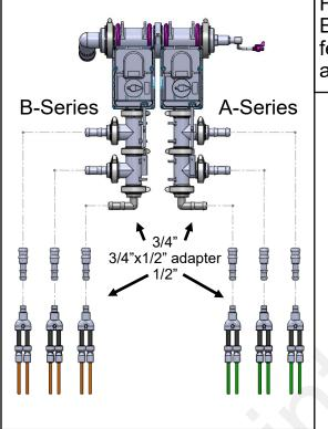
Feed section valves with 1-1/2" hose from pump. Each section valve may be split as necessary to feed the correct number of metering tube assemblies. (12 row example shown at left.)
