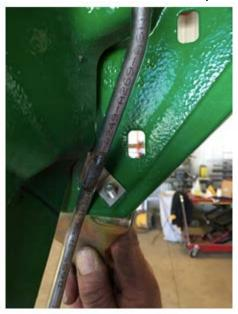
5. Tighten the disc guard nut back into place.
