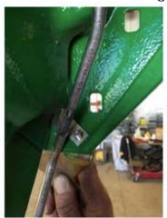
3. Slide ExactEmerge Fertilizer tube over disc bolt as shown. This bracket takes the place of two (2) shims. It is the exact width of two (2) shims.
