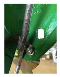
6. Align the tube so it is in the center of the seed tube guard and pinch the tab tightly around the guard with a channel lock. (We find a channel lock works the best.)
