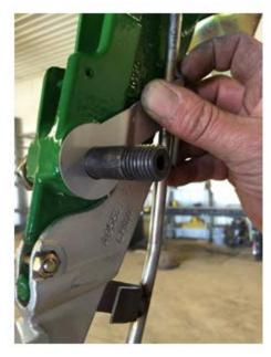
4. Slide bracket on the top of the tube over the disc guard bolt as shown.
