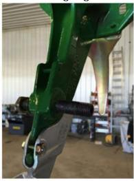
2. Remove nut holding on the disc guard.
