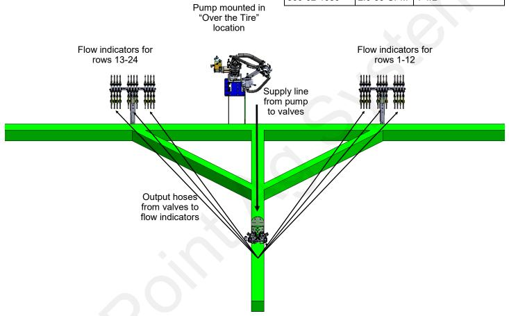
Valves A1 and B1 both feed the pre-assembled metering tube set which goes to the same set of flow indicators.
