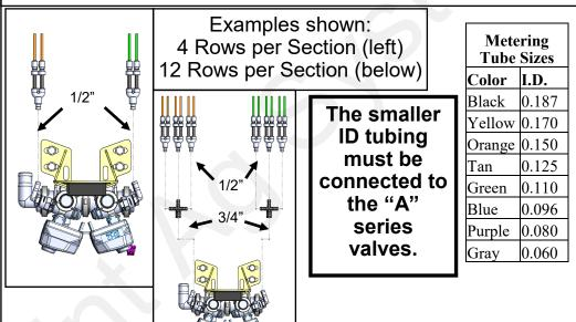
Dual metering tube comes pre-assembled in 3, 4, or 6 row assemblies. 1/2" hose barb ends go to the section valves, 3/8" tubing goes to flow indicators.
