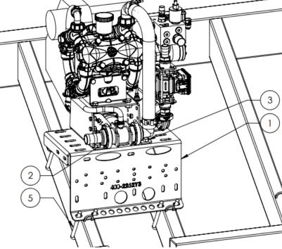
Use four (4) 1/2" x 1" hex head bolts and flange nuts to mount PumpRight pump unit to 400–2262Y3 bracket.
