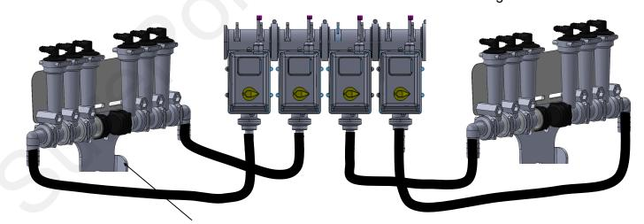
NOTE: Another option is the flange can face forward so the T-Bracket could be mounted on the front side of a bar.
