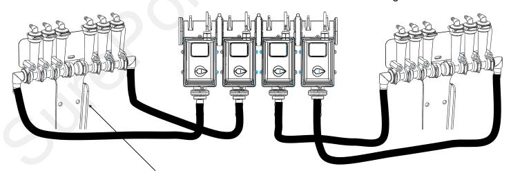
NOTE: Another option is the flange can face forward so the T-Bracket could be mounted on the front side of a bar.
