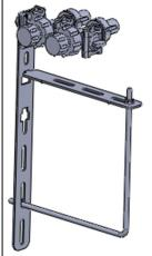
Example 3. Use the long bracket on the front of a 3x7 bar (vacuum tube on some planters). Mount the check valve hanging forward of the bar. The supply line will run directly over the bar. The excess bolt and bracket length can be cut off.
