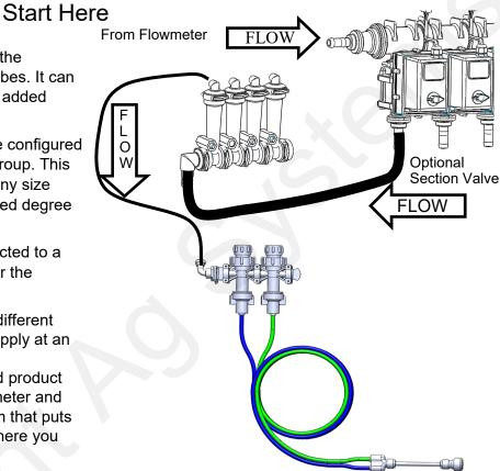
SurePoint dual metering tube plumbing kits are a great way to plumb a planter to apply starter fertilizer or high rate applications. They'll also work on other implements when applying low or high rates of fertilizer.
