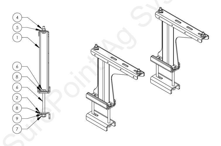
SurePoint Accelerator (55, 110 and 155 gallon) or Catalyst<sup>TM</sup> (55 and 100 Gallon) tanks can be mounted above and offset from a toolbar using this z-mount bracket. This kit attaches to 5" - 7" wide toolbars. The kit includes  $3/4" \times 9"$  bolts to work with a 7" tall bar.
