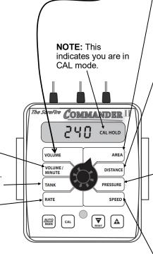
DO THIS -- WIDTH CAL: Enter the /width of each fertilizer or chemical section of your implement. For a single section system, set Section One to the full implement width in inches. For example, for an 8 row 30" implement, set Section One to 240 inches. To set the section widths the Run/Hold Switch has to be in Run and the Section Switch must be ON. If using a single section implement, set Section 2 and 3 to ZERO.
