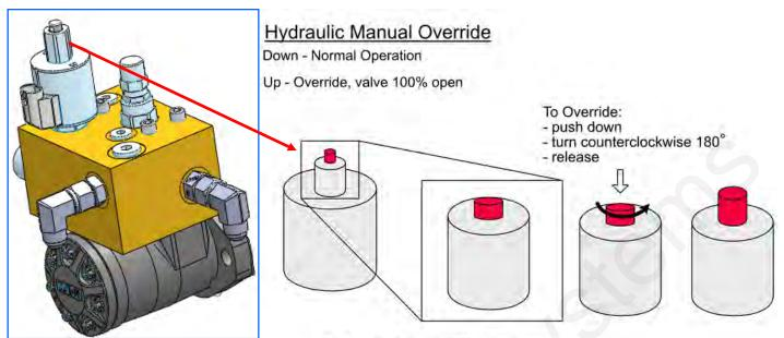
Manual Override - Override will completely open valve, so turn down the hydraulic flow in the cab.
