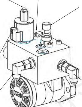
Bypass Valve—Remove the cap to access a bypass needle valve. This valve is shipped from the factory closed. The only case when valve should be open is when running in series with other hydraulic motors.
