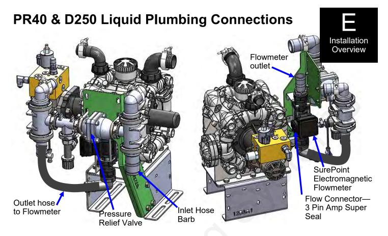
**Inlet:** The PR40 and D250 PumpRight are shipped with a 2" inlet hose barb. Attach this to the hose from your supply tank and strainer. A 2" 90 degree hose barb is included and can be substituted.
