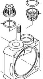
D70 - D115 Valves are on same side of head. Valves should pop out with slight screwdriver pressure.
