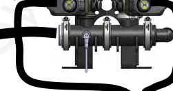
This is usual ly 3/8" hose. Maximum recommended length is 20 feet and lengths do not need to be equal.
