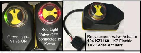
This is a 3-way valve. If product not flow when valve is ON, either move the outlet hose to the other port, or remove actuator and rotate valve ball 180°, and replace actuator.
