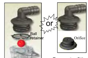
If using a metering orifice in the flow indicator, the orifice replaces the ball retainer. If not using an orifice here, the ball retainer must be in place.
