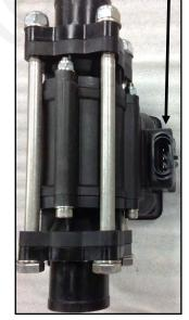
Amp SuperSeal 3-pin connector Use adapter 201-17842 to connect to 3-pin MP harness
