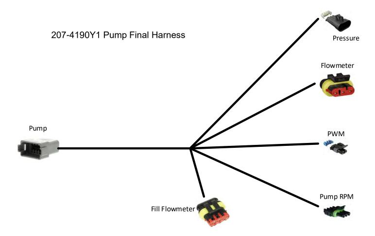
Note: On the Trimble Field-IQ module, the Pump Final harness MUST have a Yellow and a **Green** wire on the PWM connector. 207-3461Y2 or 207-3462Y2 will NOT work.
