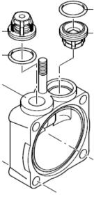
D70 - D115 Valves are on same side of head. Valves should pop out with slight screwdriver pressure.
