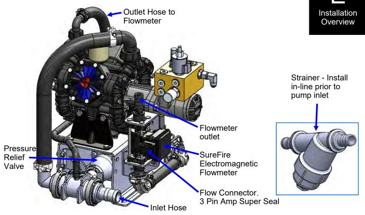
**Inlet:** The PR17 and PR30 PumpRight are shipped with a  $1 \frac{1}{2}$ " inlet hose barb. Attach this to the hose from your supply tank and strainer. A  $1 \frac{1}{2}$ " 90 degree hose barb is included and can be substituted.
