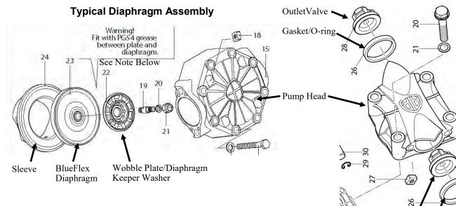
NOTE: A multipurpose grease is fine to use for applying in between the Diaphragm and Wobble Plate/Washer
