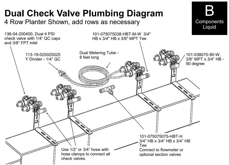
This is a general diagram showing the dual check valve assembly mounted on a planter toolbar. The check valve and bracket are very flexible in their mounting. The check valve can mount behind, directly over, or in front of the toolbar. The check valve can be put in the bracket facing up & down or sideways (shown). In addition, the steel bracket could be rotated 90 degrees and clamp around the bar. The multiple slots in the bracket are used to mount to any tube 7x7 inches or smaller.
