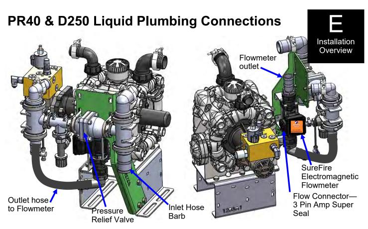
inlet hose strai subs inlet hose strai subs inlet man anyv mou to th Outi hose to th The prior flown Pres
