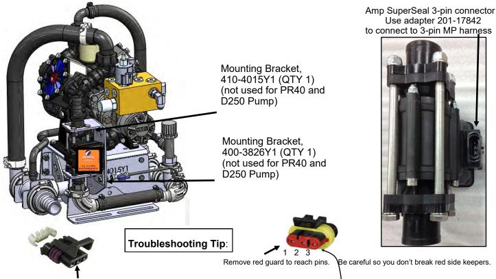
**3-pin MP Tower A- Signal B- 12V Power C- Ground** (See the next) page for more flowmeter tips) **3-pin AMP SuperSeal 1– Ground 2– 12V Power 3– Signal**
