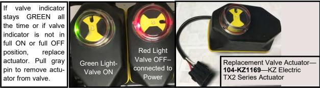
*This is a 3-way valve*. If product will not flow when valve is ON, either move the outlet hose to the other outlet port, or remove actuator and rotate valve ball 180°, and replace actuator. Product should flow through the port closest to the Indicator light when the valve is open (green).
