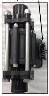
Remove red guard to reach pins. Be careful so you don't break red side keepers.
