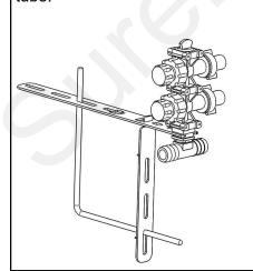
Example 2. Use the long bracket on the rear of a bar. The check valve is mounted over the top of the bar. The supply line would run above and behind the bar. The short bracket is placed in the notch to mount the
