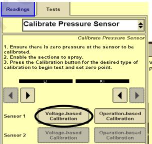
Tip: If the system has been running, there may be pressure in the system due to the check valves. In that case, simply unplug the sensor while this setup is being done so it will calibrate the zero point correctly.
