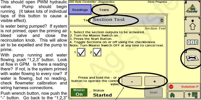
Go to Step 2 on the next page when you can increase and decrease the GPM reading using the + and - buttons.
