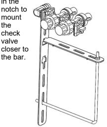
Example 3. Use the long bracket on the front of a 3x7 bar (vacuum tube on some planters). Mount the check valve hanging forward of the bar. The supply line will run directly over the bar. The excess bolt and bracket length can be cut off.
