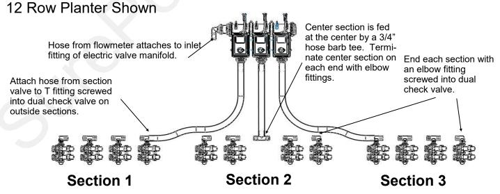
For a **2 section plumbing system**, omit the center section and plumb similar to the outside 2 sections.
