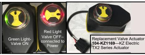
This is a 3-way valve. If product will not flow when valve is ON, either move the outlet hose to the other port, or remove actuator and rotate valve ball 180°, and replace actuator.
