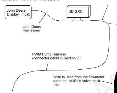
3/4" or 1" hose typical from each LiquiŚhift valve to each LiquiShift tube assem-
