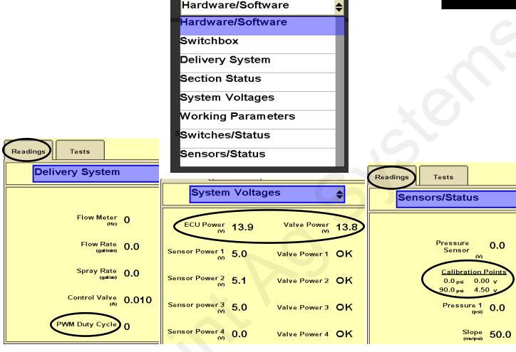
Check the operation of the **flowmeter** here on the Delivery System screen.
