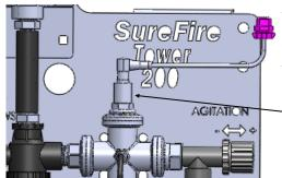
setting up sensor as Sensor 2. If still no voltage, check harnessing by using a AA or AAA battery and connecting Pin A of the Pressure connector to the (+) end of the battery, and Pin C to the (-) end of the battery. It should show 1.5 v and 30 PSI on the screen.
