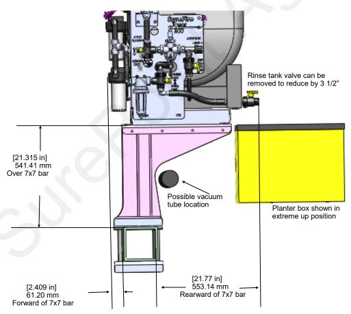
This mount kit includes two welded brackets to mount any of the 3 sizes of accelerator tanks above and offset from the 7x7 planter toolbar as shown.
