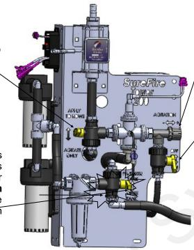
Agitation Adjust Valve: RECIRCULATION KNOB This valve adjusts how much flow returns to the tank while working in the field. Normally closed. If needed, start with a quarter turn.
